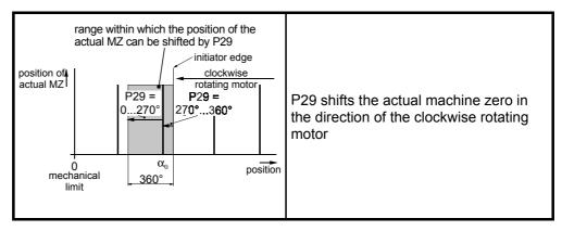
Example 2:  $\alpha_0 = 90^{\circ}$ ; clockwise rotating motor away from the direction of the mechanical limitation travel
